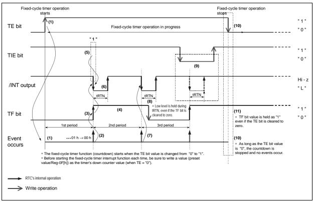
\* Before starting the fixed-cycle timer interrupt function each time, be sure to write a value (preset value/Reg-0F[h]) as the timer's down counter value (when TE = "0").
